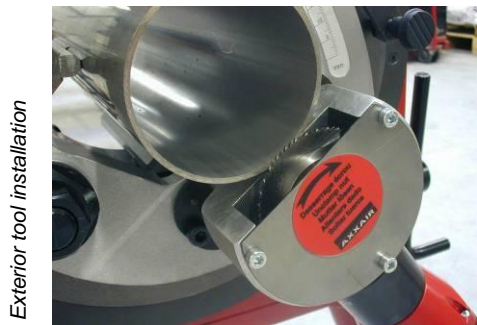
Tool installation near the jaws
